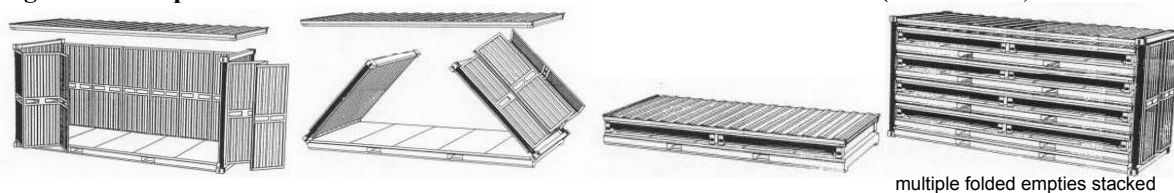
Figure 3 Concept of the foldable container of Holland Container Innovations (Source: HCI)
